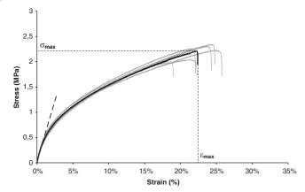
**Figure 1.**Stress-strain curves for the material made from a wheat-flour containing 6.5% proteins (w/w). Grey curves show the full set of measurements, black curve is the calculated mean curve. – – –: tangent at origin of the mean curve.
