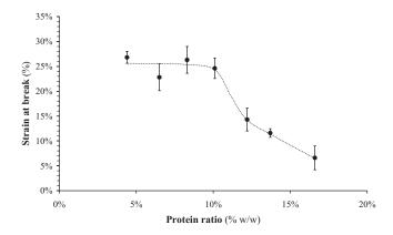
Figure 3. Evolution of the strain at break as a function of protein ratio in wheat flour (The curve is merely drawn to guide the eye and has no theoretical basis).
