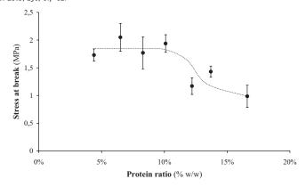
**Figure 2.**Evolution of the stress at break as a function of protein ratio in wheat flour (The curve is merely drawn to guide the eye and has no theoretical basis).
